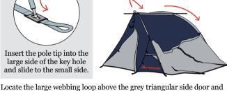
insert the ends of the short black pole into the eyelet as shown in the diagram (B).
